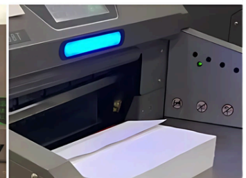
Safety photoelectric indicator light
